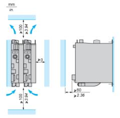
LXM32•U45M2, •U90M2 and LXM32•U60N4 servo drives are cooled by natural convection. LXM32•D18M2, •D30M2, LXM32 •D12N4, •D18N4, •D30N4 and •D72N4servo drives have an integrated fan.
